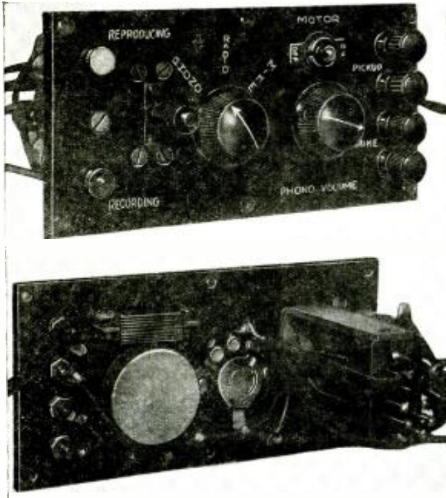
Fig. A, above; Fig. B, below The front and rear views of the panel of the home-recording control unit.
